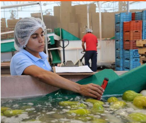
Water tanks at the packinghouse are used to remove latex, dust, dirt, and leaves from the mangos. The hydrothermal tank serves to eliminate the presence of the fruit fly, and the hydrocooling tank rapidly cools the mangos so they can be packed.
